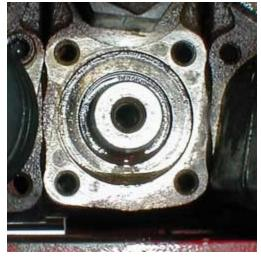
Remove the valve cover and clean out the old seal.
