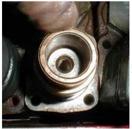
Next, slide in the smaller bushing and use it to push in the seal. The larger bushing keeps the lip from catching.
