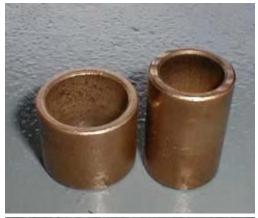
This is a trick I learned working at the local Toro Distributors. It's using these two bushings to help install the seals in the valve bank.
