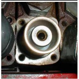
Instead, slide the larger bushing over the seal. Sometimes I have to start with the seal inside the bushing.
